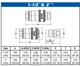
\*Hex dimensions are taken from flat of hex and not across corners. Hex may be substituted with round stock. Hex column would then indicate dimension taken across wrench flats. Decimal dimensions are  $\pm$  .06 in. (1.5mm)
