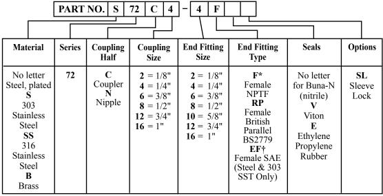
\*316 stainless steel construction supplied with female NPSF threads
